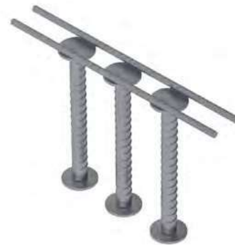
The element with 3 anchors
