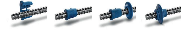
Installation of HyDra Swell Ring Connector Ø15, where the connector is locked onto the tie rod using the integrated locking strap.
